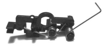
With all pieces back in place, test the operation of the PLAY key and modify the spring if necessary. Once things are working OK, put the tape deck back together and enjoy your Pianocorder for a few more decades!
