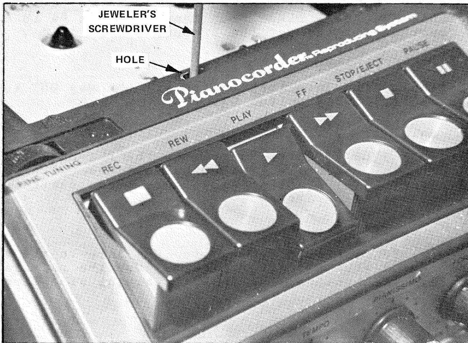
FIGURE 9-3 Insert the screwdriver through the hole in the Recorder case.
