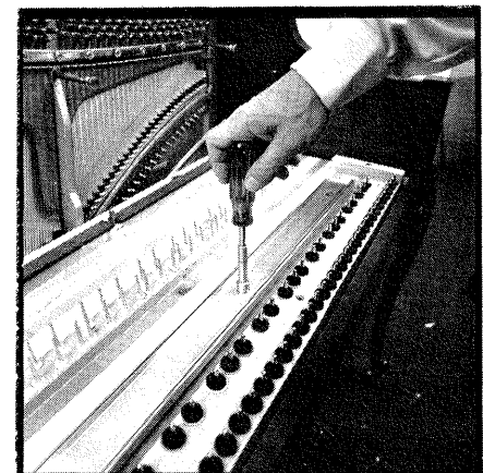
FIGURE 3-21 Lower the rail to the keybed.
