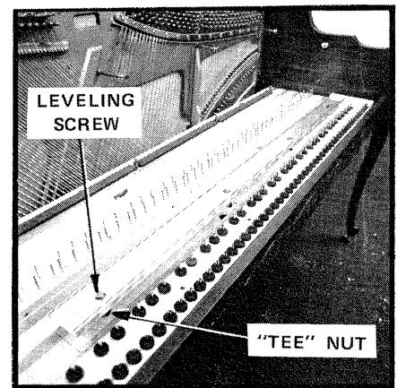
FIGURE 3-20 Center the Leveling Screws in the "Tee" Nuts.
